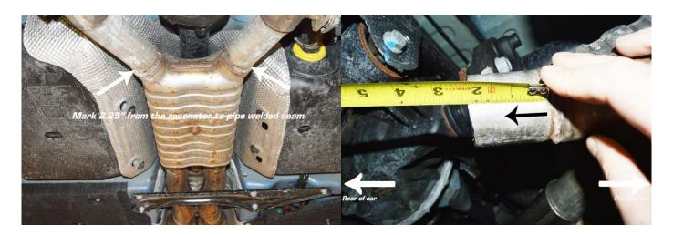
Step #1: Measure 2 ¼" from the seam where the outlet portion of the resonator and tube are welded.
