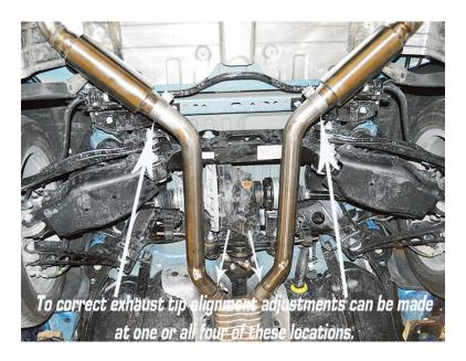
**NOTE:** Adjustment of tip can be made by sliding the under axle pipes or muffler assemblies in/out and rotating at each clamp joint.
